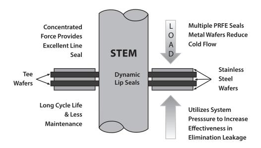
Dyna-Pak® provides superior sealing performance while reducing maintenance costs. Consisting of alternate wafers of TFE and metal spacers, stem leakage is virtually eliminated while the problems associated with TFE cold flow are minimized.
